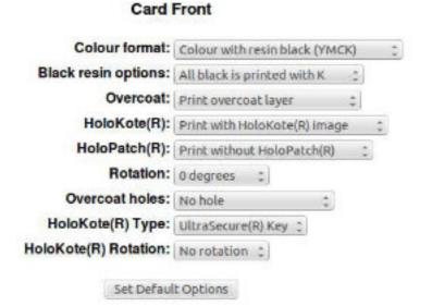
Colour format – determines the colour composition of the printed image, the printer can use the colour panels of the printer ribbon to make coloured cards (YMC), any black (such as text) can be printed using the black resin ribbon panel (K)
